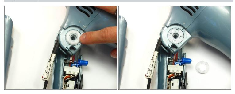
• Remove the inner white disk piece by gently pulling it out with your finger nail.
