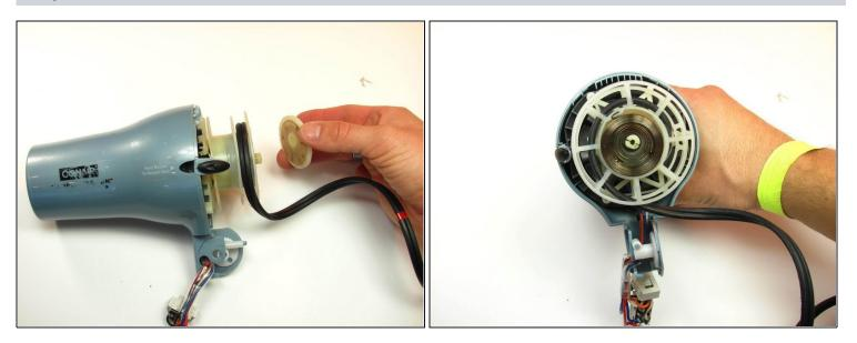
• Take off the white cap that covers the heating coil. You will see a wound up piece of metal (cord retracting coil) underneath once the cap is removed.
