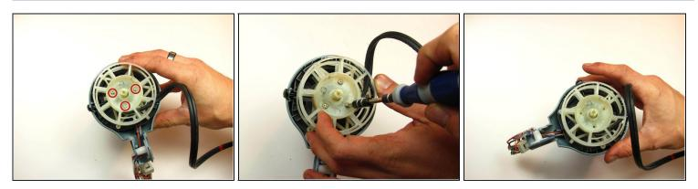
Once the coil is removed, unscrew the three 11 mm long Phillips #2 screws underneath to remove the retracting wheel.
