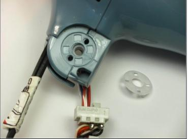
• Remove the inner white disk piece from the base of the dryer head by gently pulling it out with your finger nail.
