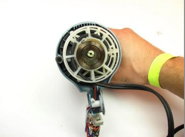
• Take off the white cap that covers the heating coil. You will see a wound up piece of metal (cord retracting coil) underneath once the cap is removed.
