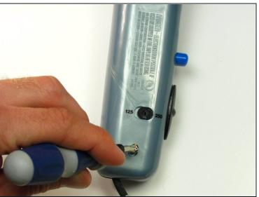
Unscrew the two 18 mm long Phillips #2 screws on the side of the hair dryer.
