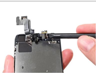
Use the flat end of a spudger to gently peel the front-facing camera portion of the cable away from the display assembly.
