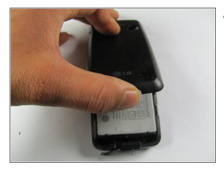
Remove the phone's back cover by placing your thumb the above charging port, located at the bottom of the phone, and sliding the back cover upward.
