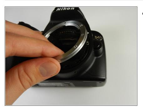
Once all 6 screws are removed, the lens mount can be gently removed from the camera.
