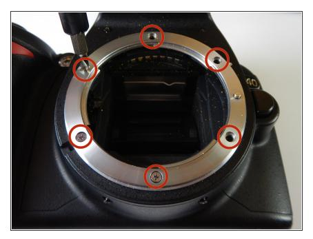
Remove the six 5.0 mm Philips #0 screws that go through the lens mount.
