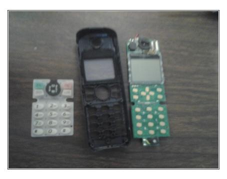
Take out the old rubber keypad and replace with a new one.
