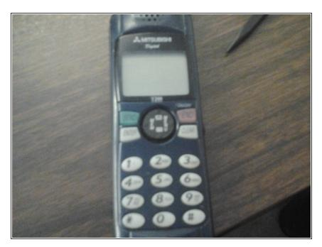
Begin disassembling the phone by removing the back of the phone and the battery.
