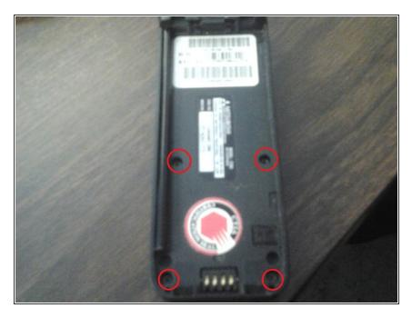
Remove the back plate by removing the 4 screws in the back plate using an appropriately sized Philips screwdriver
