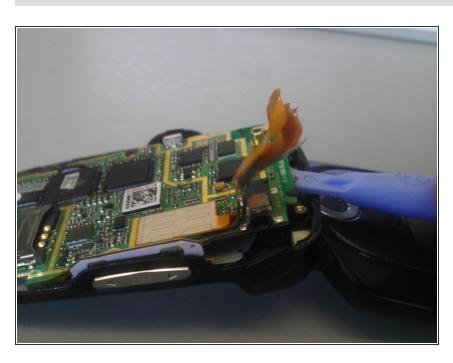
Using a small plastic opening tool, remove the motherboard.
