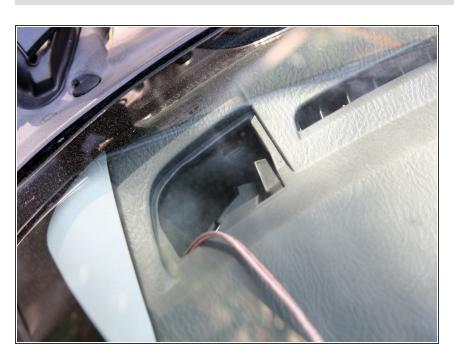
Start routing your tweeter speaker cable from through the hole on top of the dash.
