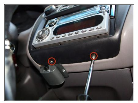
Use a #2 Philips screwdriver to remove the two screws holding the center of the dashboard in place.
