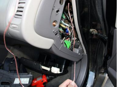
Perform the same speaker wire routing on the passenger side. The procedure should be very similar.
