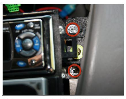
Remove the four screws (two on each side) holding the <u>double-DIN</u> stereo frame in place using a #2 JIS screwdriver or 8mm socket wrench.
