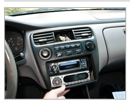
Now, gently pull the bottom of the center console towards you. Don't yank it out, there's two more connectors holding it in place.
