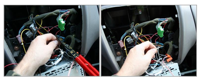
Use a pair of wire cutters/strippers to strip a portion of the both the tweeter speaker wires, as well
