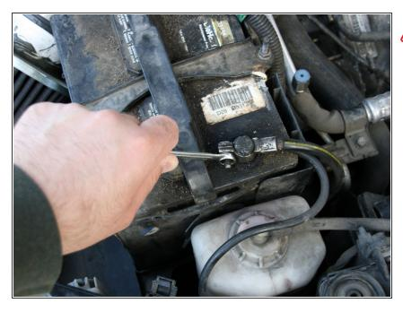
Before going any further: disconnect the battery. I keep a 10 mm wrench in my center console specifically for this purpose.
