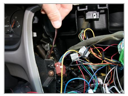
Dig deep through your center dash (while being careful not to snag your hand on any of the wiring) and pull out the speaker wire you were routing.
