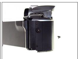
Remove the remote control socket cover.
