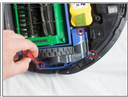
Find the blue wheel at the bottom of the Roomba, and unscrew the three captive screws holding it in place using a Phillips #1 screwdriver.
