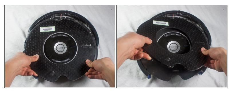
• Grab the faceplate by the outer edge and pull upwards, freeing the center friction locks in the process.
