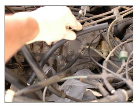
Attach a 12" or so length of 5/16" fuel line on the supply and return lines, using appropriately sized barbed fittings to create hose extensions to make it easier to insert the hoses in your temporary "fuel tank".
