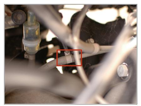
To begin, loosen the clamp on the rubber fuel hose that connects to the supply hard line. The supply line is the lower of the two, where the hose goes to the clear plastic pre-filter.
