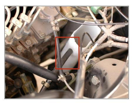
You'll need to create a small temporary "fuel tank" for the diesel purge. Any plastic bottle will work. You'll want to cut a hole in it for the supply hose so that the hose can reach the very bottom of the "tank".
