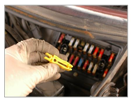
You can use a little plastic fuse remover/installer tool like shown to pull out any questionable fuses for further inspection and replacement.
