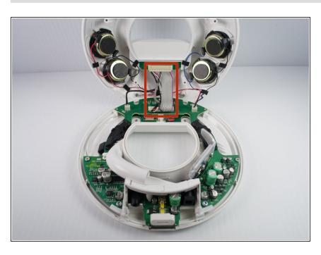
Disconnect the ribbon cable connector from the top half of the device by pulling outward and parallel to the connecting pins.
