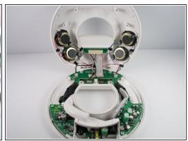
Open the device along its seam.
