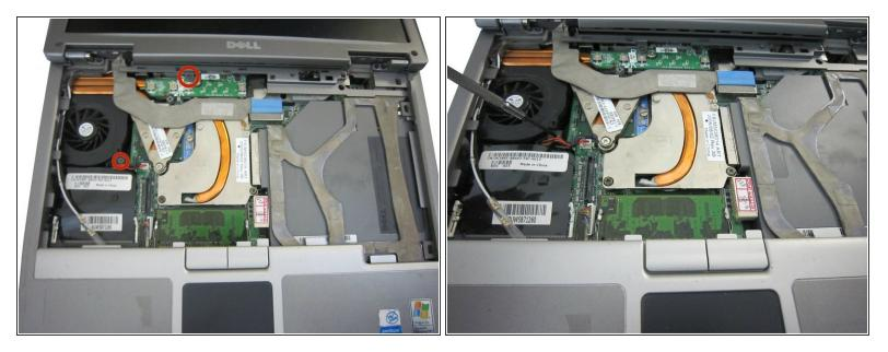
Remove the two 3.9mm Philips #1 screws from the case.
