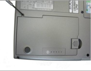
Remove the sixteen 3.9mm Philips #1 screws from the back.
