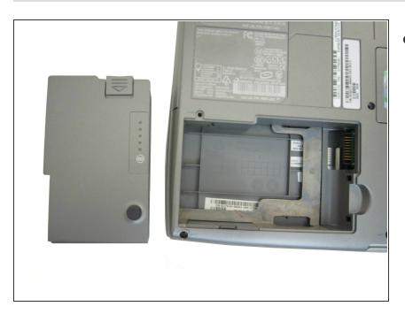
Remove the battery from its compartment.
