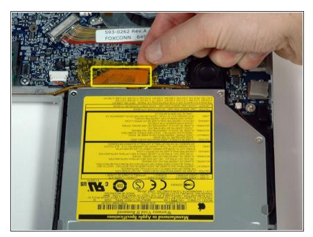
• Disconnect the orange SuperDrive ribbon cable from the logic board, removing tape as necessary.
