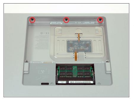
Remove the three Phillips screws in the battery compartment near the latch. Apple was nice enough to tilt these screws at a slight angle to make them easier to remove. On the A1261 these screws have 4 mm diameter heads rather than the 3 mm heads on the body screws.
