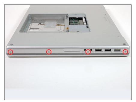
Rotate the computer 90 degrees again and remove the four Phillips screws from the side of the computer.
