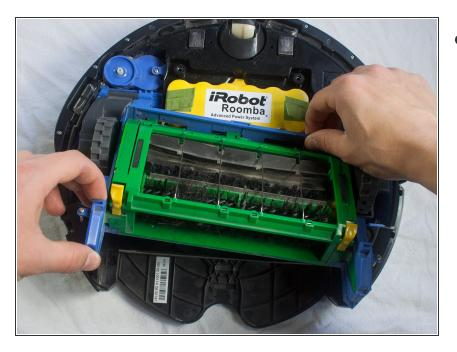
Grab the brush case and pull upwards to remove.
