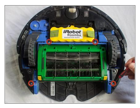
Use a Phillips #1 screwdriver to loosen the 4 captive screws around the case.
