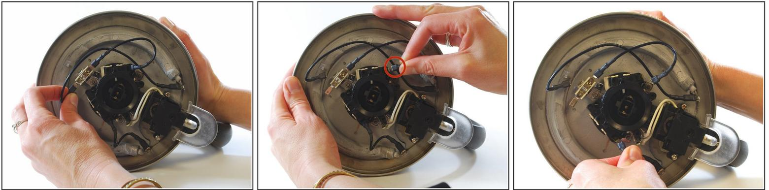
☞ Take note of how the wires connect to the components to aid reassembly.
