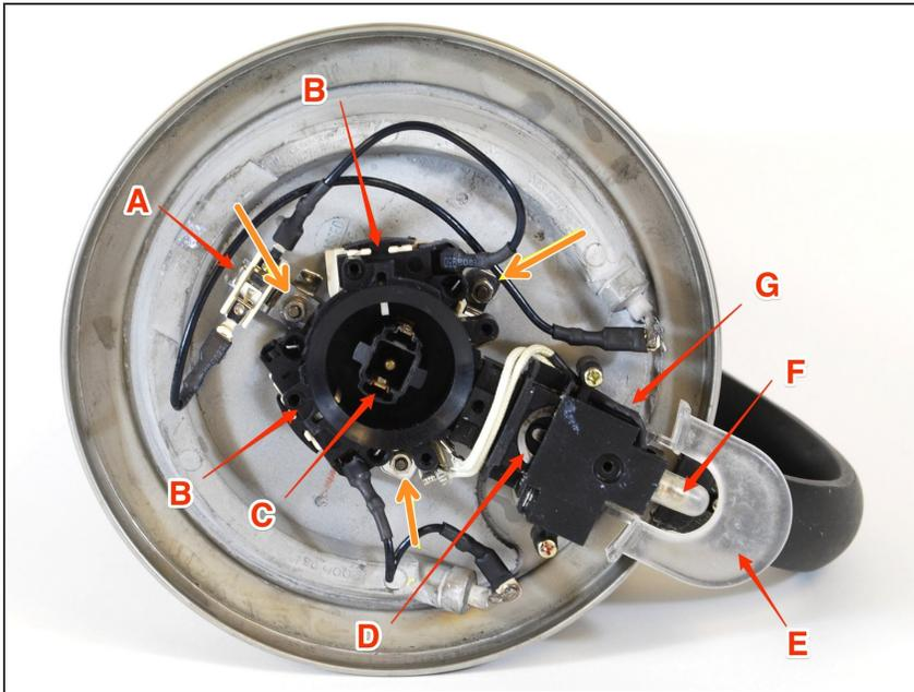
**i** Now that you have removed the bottom from the kettle, identify all of the parts. The ORANGE arrows point to the posts for mounting the control circuit components. The RED arrows point to the following parts:
