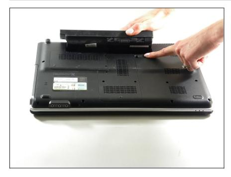
• While holding the release, lift the battery away from the battery bay.
