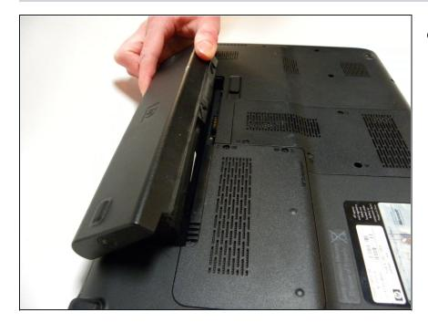
Place the new battery into the battery bay, making sure the connectors are lined up so the battery can click into place.
