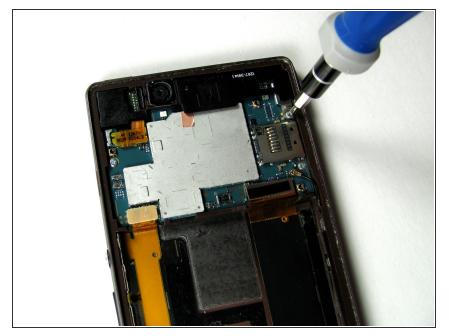
• Remove the one 3 mm screw with the Phillips #000 screwdriver. The screw is located at the top right corner of the motherboard. The motherboard is the green/silver circuit board at the top of the phone.
