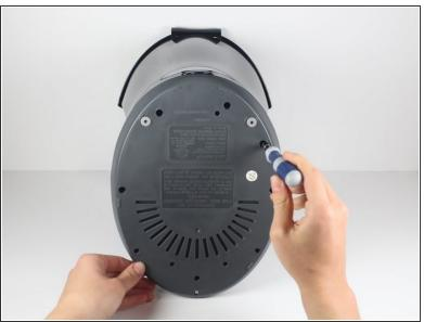
Remove the eight 11 mm screws that secure the base of the machine with a Phillips Head #2 screwdriver.
