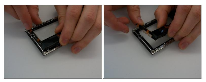
• The buttons, built-in speaker, and rumble device are all contained in a black plastic assembly. This assembly simply snaps into place at the top of the case. Lift up gently to remove it from its place.
