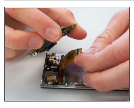
Finally, disconnect the ribbon cable on the bottom of the circuit board.
