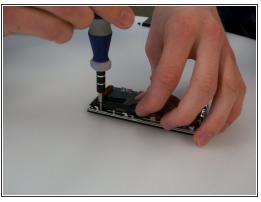
Remove the six screws (Phillips #000, 2.3 mm long) holding the screen frame to the front of the case. As the picture shows, one of them is hidden under the black speaker/rumble assembly.
