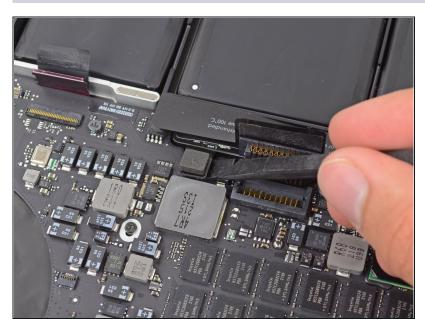
Use the flat end of a spudger to pry the trackpad ribbon cable connector up out of its socket.
