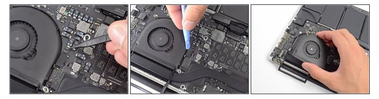
• Use the tip of a spudger to flip up the retaining flap on the left fan ribbon cable ZIF socket.
