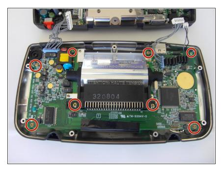
Unscrew the 8 Phillips screws from the logic board.
