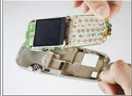
Gently remove the logic board and LCD screen from the back cover of the phone.
