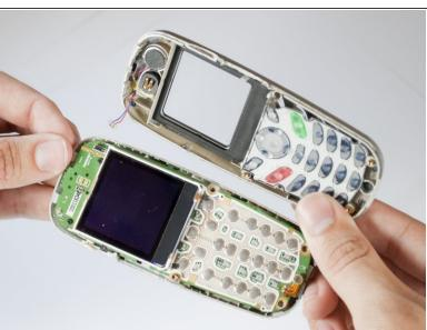
Using your nails, tweezers, or any precise grabbing tool, pinch the antenna wire connector (clear plastic plug) and pull gently. It should pop out rather easily.
