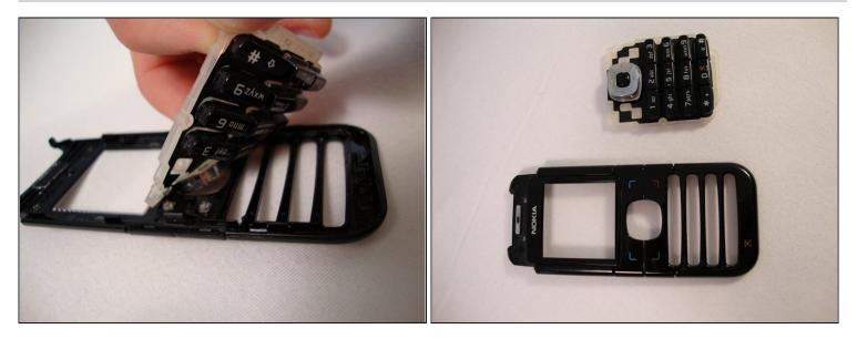
• Remove old keypad and replace it with new keypad.
