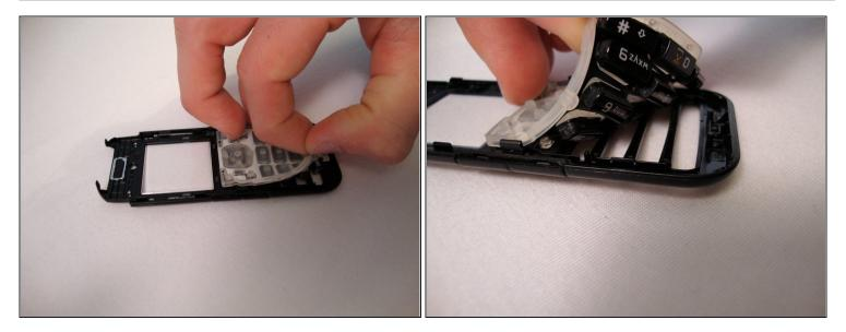
• Gently pull the rubber away from the front screen and the buttons will detach from the plastic case.
