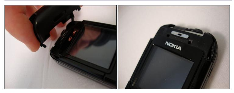
• After removing the top cover, turn the phone over so the screen is facing upwards.
