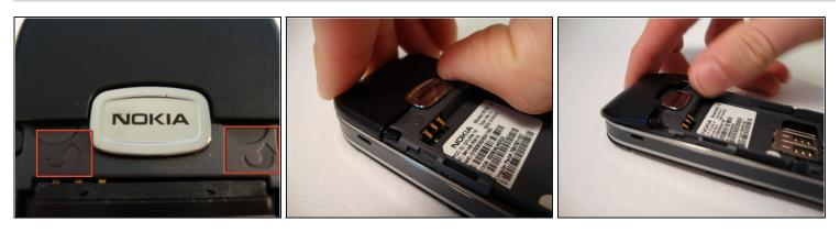
• Insert your two fingers under the two tabs found at the top of the phone underneath the black casing, then pull the casing up and slide it out slowly.
