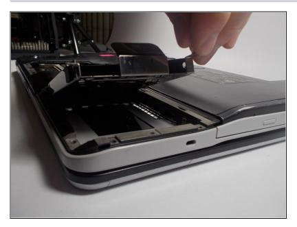
Carefully remove the hard drive from the panel in the bottom right-hand corner of the laptop.
