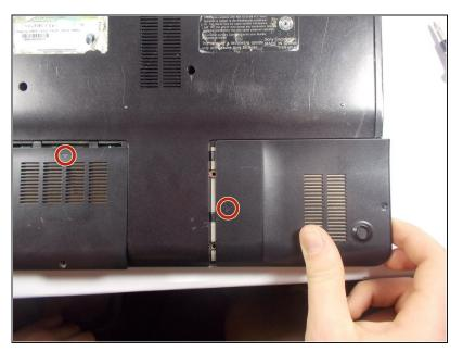
Remove the two panels in the bottom right-hand corner by sliding in the direction of the arrows imprinted on the panels.
