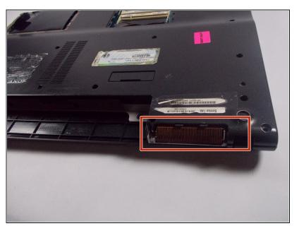
Remove cover in the top left side of the laptop next to the battery by pulling it outwards.
