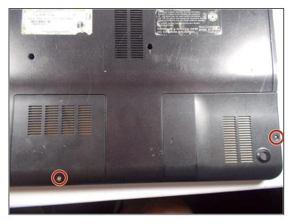
Remove the highlighted screws from the panels in the bottom right-hand corner of the laptop using the Phillips #0 Screwdriver.
