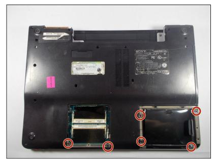
Remove the highlighted screws underneath the removed panels using the Phillips #0 Screwdriver.
