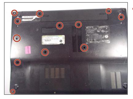
• Remove the highlighted screws from the back of the laptop with a Phillips #0 Screwdriver.
