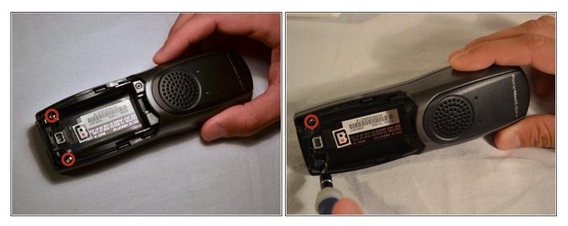
Remove the two 11mm screws inside the battery storage compartment using Phillips #1 screwdriver (located near the very bottom of the phone)
