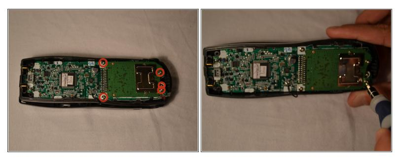
Carefully remove the middle two 7mm screws, the outer top 9mm screws, and the top middle 7 mm screw that hold the logic board to the front shell of the phone casing using the Phillips #1 screwdriver
