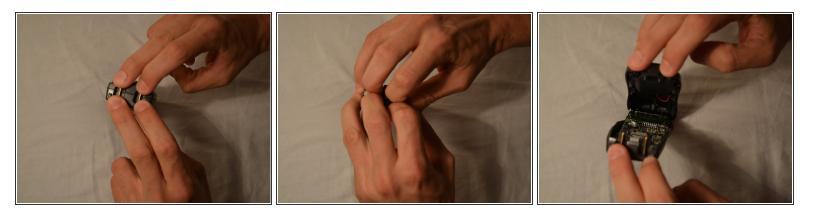
Gently open phone casing along the seam at the bottom of the phone using index and middle fingers of both hands
