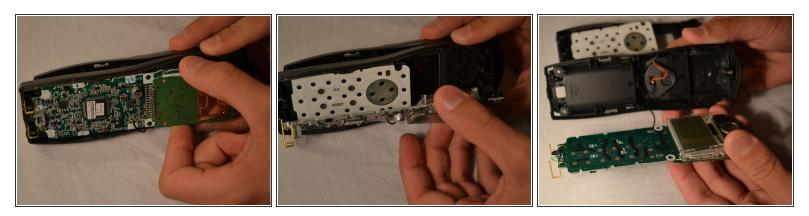
• Using index finger and thumb, carefully remove the circuit board from the front shell of phone
