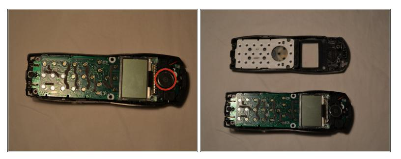
Place circuit board gently on the back shell with the earpiece facing up
