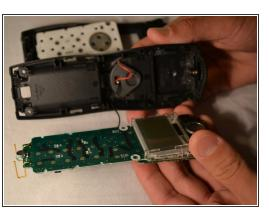
Using index finger and thumb, carefully remove the circuit board from the front shell of phone
