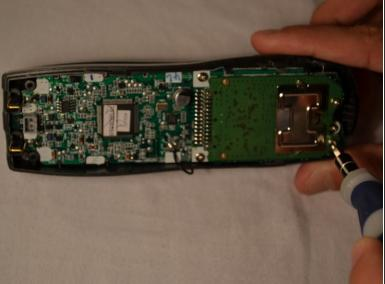
Carefully remove the middle two 7mm screws, the outer top 9mm screws, and the top middle 7 mm screw that hold the logic board to the front shell of the phone casing using the Phillips #1 screwdriver
