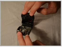
Gently open phone casing along the seam at the bottom of the phone using index and middle fingers of both hands
