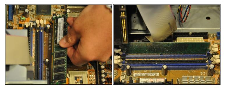
• Pull RAM card vertically out of slot.
