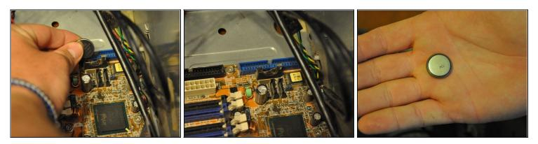
• Pull battery, in a rolling motion, out of its slot.
