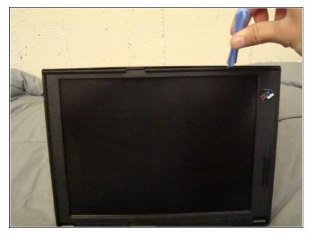
Insert the plastic opening tool between the front cover and back cover to pry open the screen case, then carefully pull the bezel off.
