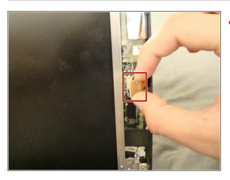
Using your fingers or an Opening Tool, detach the connector on the right side of the screen.
