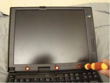
• Remove the plastic screw covers, then remove the 3 Phillips screws under them.
