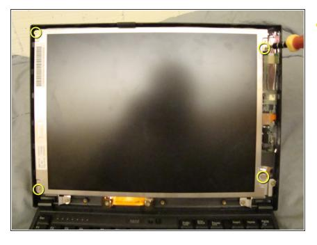
Remove the four Phillips head screws.
