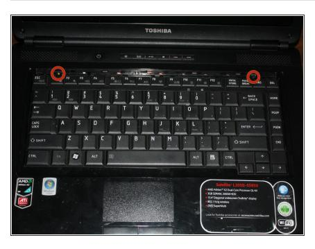
Use a phillips head #0 screwdriver to remove the two 3.75mm screws holding the keyboard in place.
