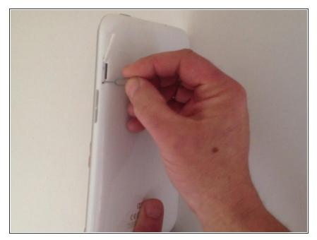
First of all you can try soft reset from the reset switch. This method does not delete the data from the tablet.
