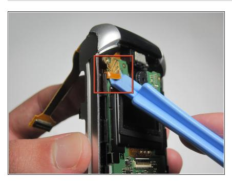
Using the iPod Opening Tool remove the yellow flex cable from the green logic board.
