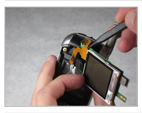
Use Spudger or hands to detach flex cable from front screen logic board
