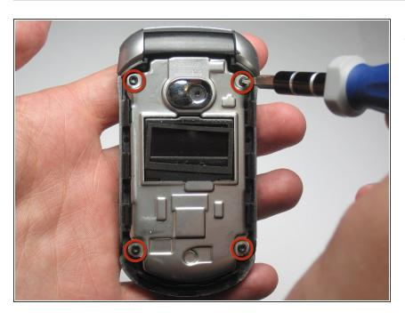
Using the T6 Torx Screwdriver remove all 4 small screws.
