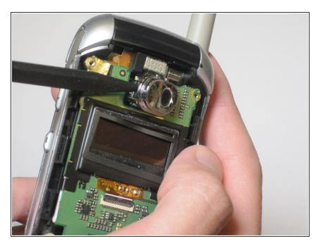
Using the spudger remove the plastic camera casing
