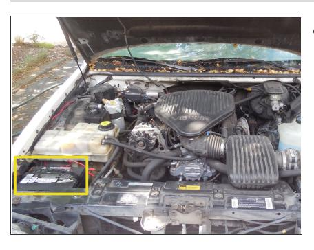
Find the battery, this is normally to the left front of the engine.
