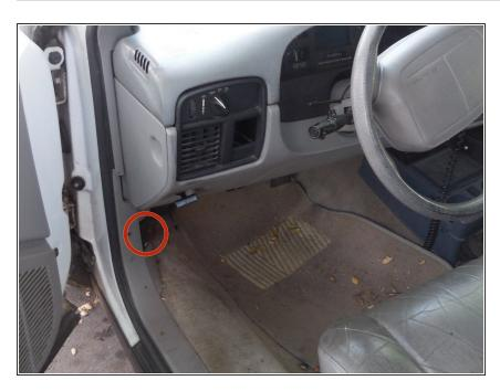
Find the hood lever, this is normally under the dash, to the left of the steering wheel.
