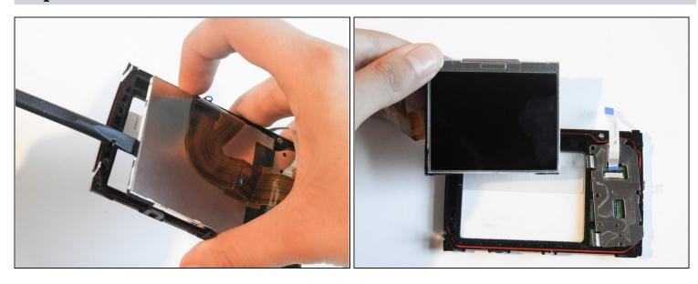
• Use the spudger to carefully pry off the LCD screen.
