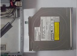
• Push to the right with your finger placed on the left side of the drive until it is completely removed.
