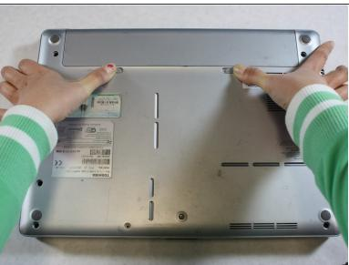
Slide both of the latches to the outside to release the battery.
