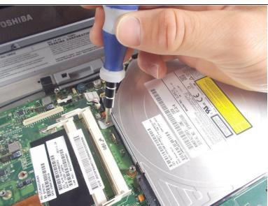
Locate and unscrew the Phillips-head #00 4.65mm screw that attaches the drive to the motherboard. It is located on the left hand side of the actual drive.
