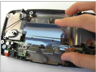
Unscrew the screws to remove the metal covering.
