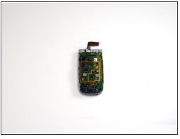
Use your fingers to detach the ribbon wire located on the top of the logic board, as shown.
