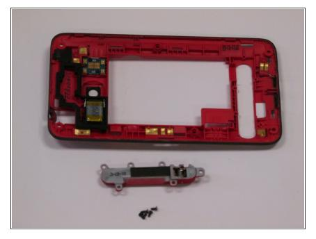
Remove the stand from the frame by lifting it out. Clear any debis causing it to be jammed, or replace with new stand.
