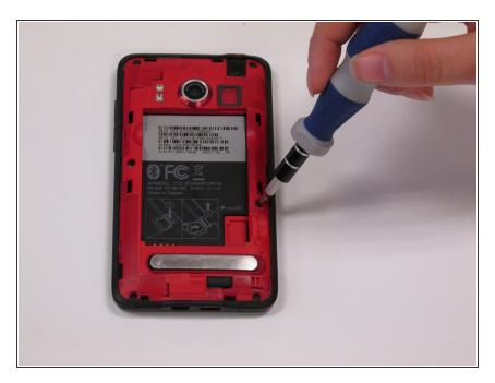
you should remove the six T5 screws holding the Inner frame in place. Be careful not to loose the screws
