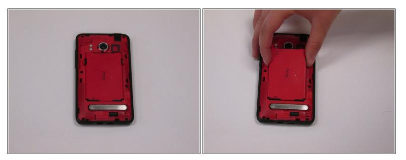
• Remove the battery from the phone by carefully lifting it out with your fingers.
