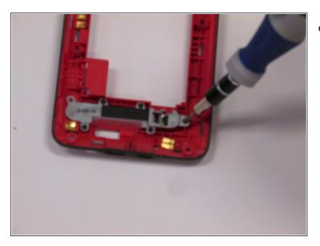
Remove the five screws that are holding the stand in place.
