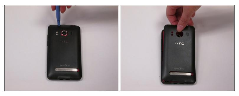
• Remove the back case of the phone with a plastic opening tool by placing the tool in the tab on the back of the phone.
