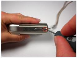
• Locate the 3 screws on the outer metal band and remove them with a #00 Phillips screwdriver.
