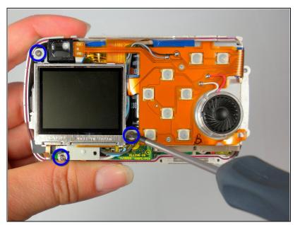
Locate the 3 internal screws holding on the front of the case.
