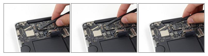
• Use the flat end of a spudger to pry both antenna connectors up from their sockets on the AirPort/Bluetooth card, and move them out of the way of the card.
