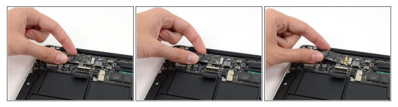
Slightly lift the free end of the AirPort/Bluetooth board and pull it straight out of its socket on the logic board.
