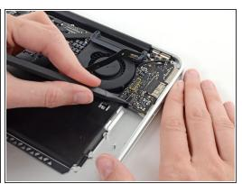
Use the tip of a spudger to carefully flip up the retaining flap on the microphone ribbon cable ZIF socket.
