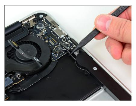
Use the tip of a spudger to de-route the left speaker cable from the notch cut into the edge of the I/O board.
