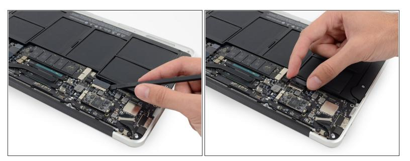
In this step you will disconnect the battery to help avoid shorting out any components during service.
