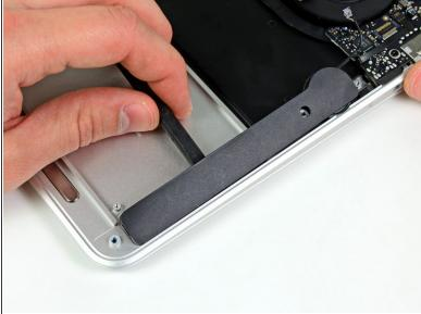
• Use the flat end of a spudger to pry the left speaker off the adhesive securing it to the upper case.
