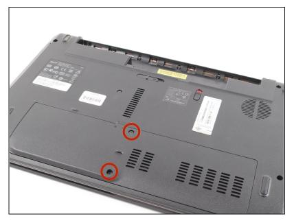
Now, locate the two screws that hold the back cover panel onto the laptop.
