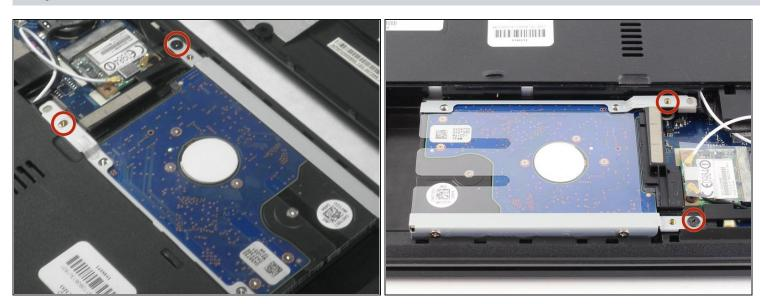
Locate the two screws that are holding the hard drive in place.
