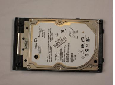
Press thumb down firmly on the hard drive and pull outwards to the side.
