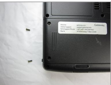
Remove the two 9 mm Phillips #0 screws from the back of the hard drive cover.
