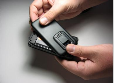
Remove the back cover by locating the slit on the bottom of the phone and lifting up.
