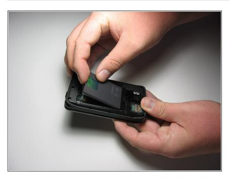
Remove the battery by lifting it out of the device.
