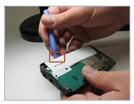
Use a blue plastic opening tool lift the motherboard out of the back cover
