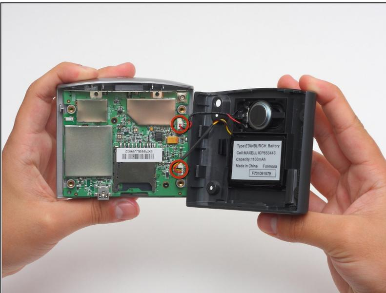
⚠ Carefully pull the back cover apart from the front cover. Be careful not to pull too hard because there are two sets of wires connecting the device.
